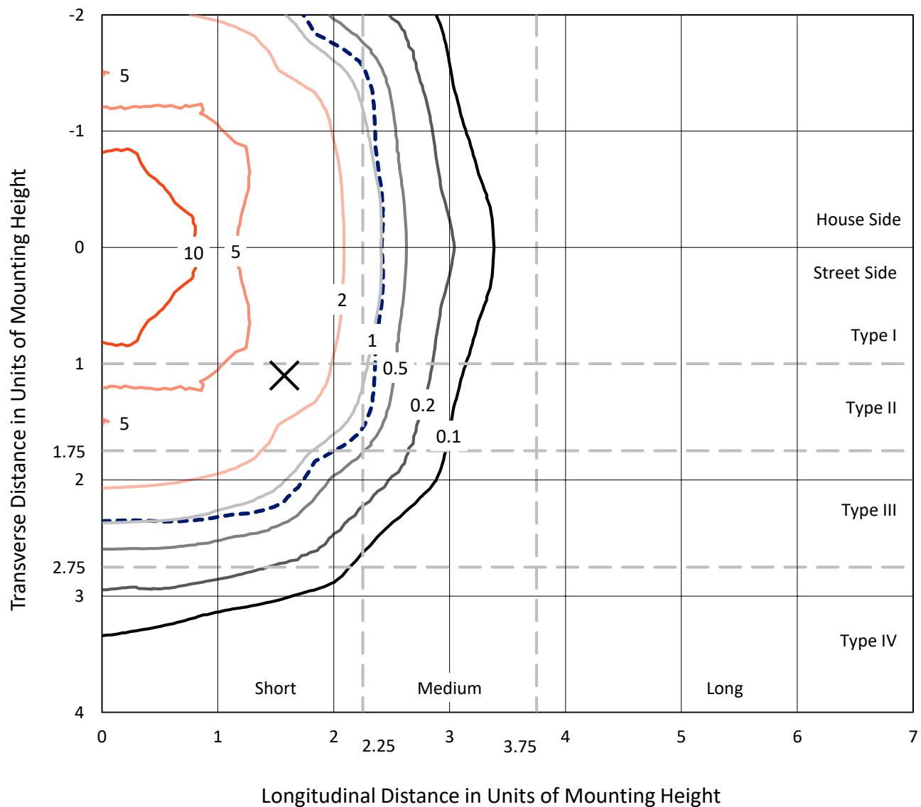
Based on 10 foot mounting height. Maximum calculated value = 19.1 fc
