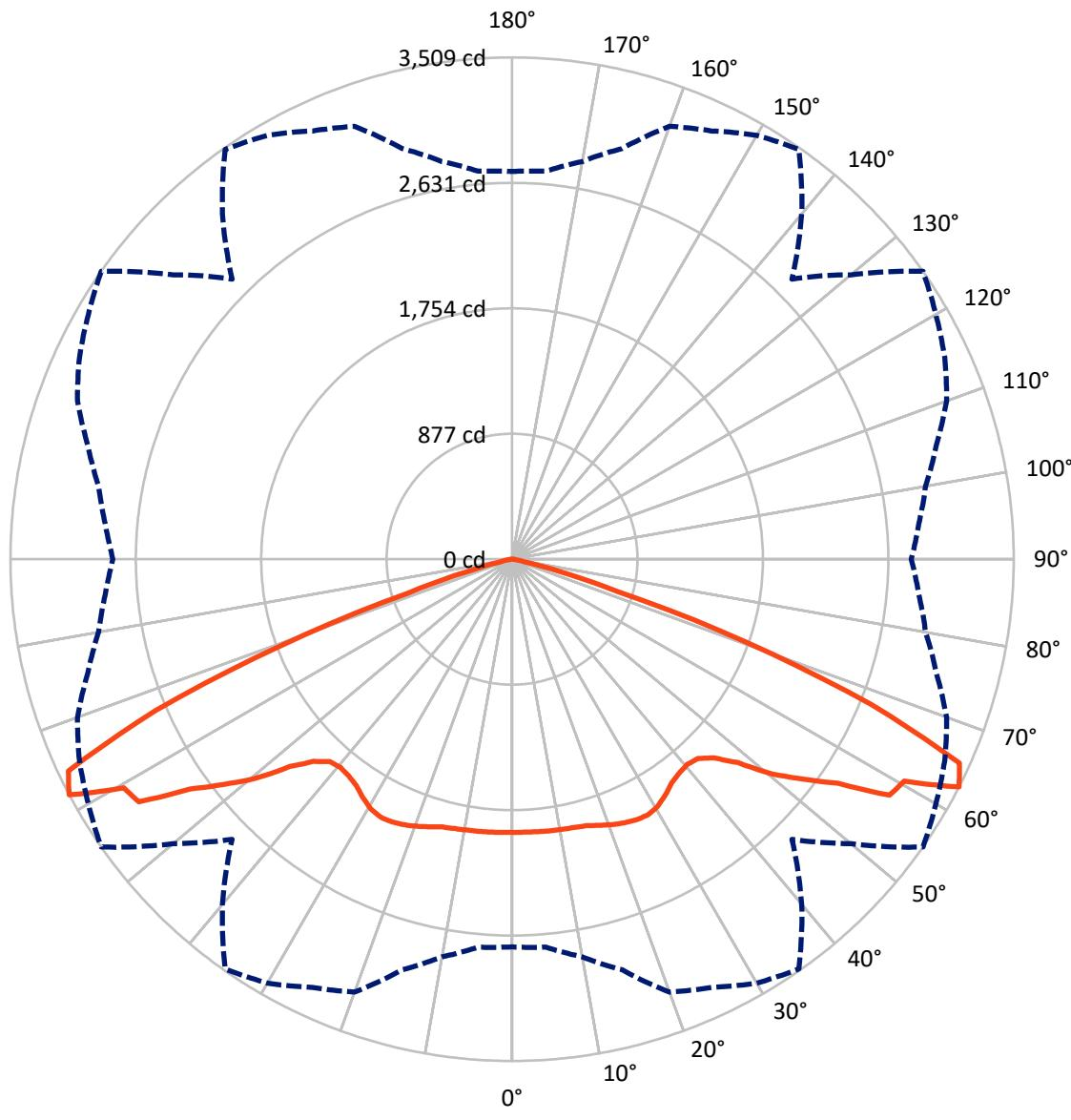
— Vertical Plane Through 55-Deg Lateral    - - - Horizontal Cone Through 62.5-Deg Vertical
